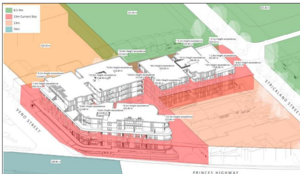
Figure 4: 3D Height Exceedance Diagram - DA-0-900 (Source: Dickson Rothschild)
