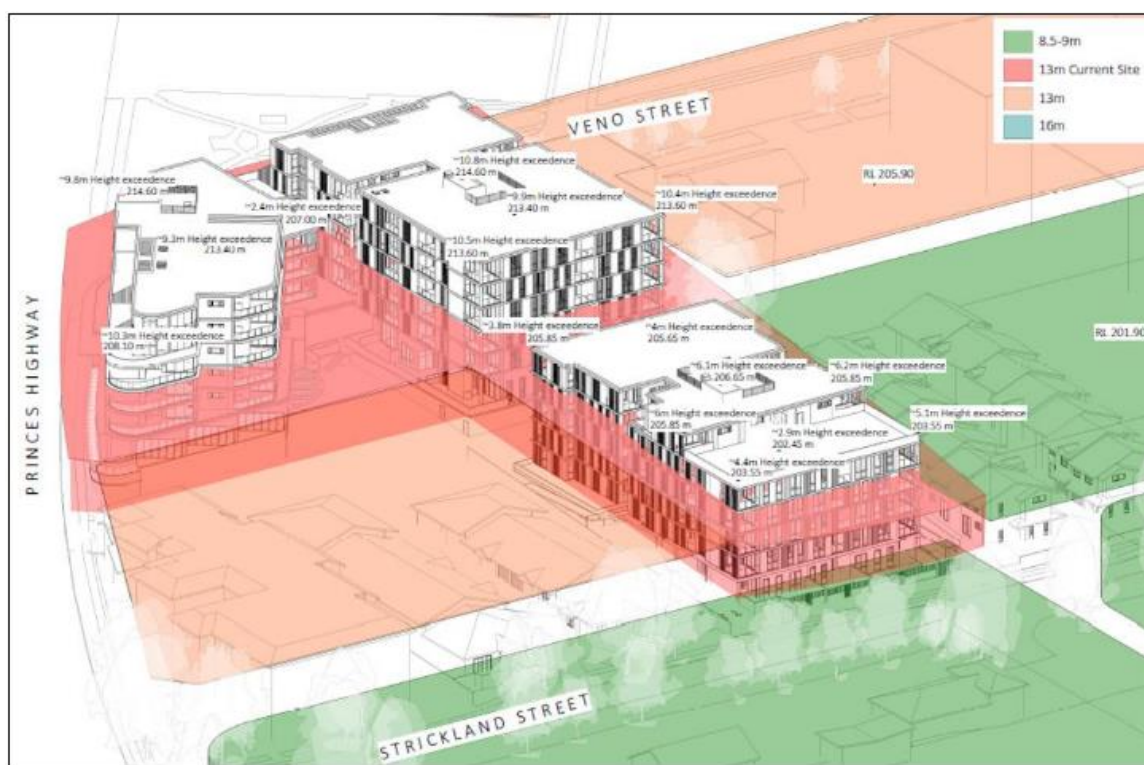
Figure 5: 3D Height Exceedance Diagram - DA-0-901 (Source: Dickson Rothschild)
